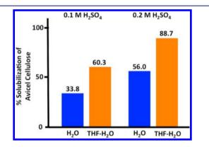
**Figure 6.** Comparison of the % solubilization of Avicel cellulose in heated batch reactions solvated in water-only or in THF–water cosolvent mixtures at two dilute sulfuric acid concentrations. The reaction temperature was 445 K and the duration was 30 min for all reactions.
