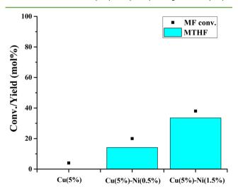
**Figure 5.** MF conversion and MTHF yield over  $Cu(5\%)/TiO_2$  and  $Cu(5\%)-Ni(0.5 \text{ and } 1.5\%)/TiO_2$  catalysts. Reactions were conducted at MF loading of 1 g, catalyst loading of 0.3 g, with 25 mL of 1, 4-dioxane as a solvent, temperature of 200 °C, 35 bar of H<sub>2</sub> (at 25 °C), and 4 h reaction time.
