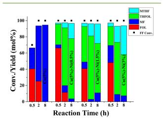
Figure 3. FF conversion and product yields as a function of reaction time on  $Cu/Al_2O_3$  and  $Cu-Ni/Al_2O_3$  catalysts. The catalyst composition is noted in the 8 h reaction time bar. All reactions were conducted at FF loading of 1 g, catalyst loading of 0.3 g, with 25 mL of 1,4-dioxane as a solvent, and at a temperature of 200 °C. The reactor was pressurized with 35 bar  $H_2$  gas at 25 °C.
