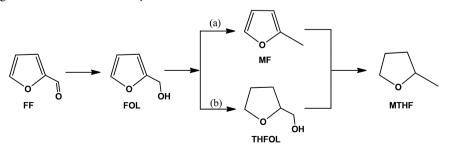
"Path (a) represents the hydrogenolysis of FOL to MF followed by ring hydrogenation of MF to form MTHF. Path (b) represents furan ring hydrogenation in FOL to form THFOL followed by further hydrogenolysis THFOL to form MTHF.
