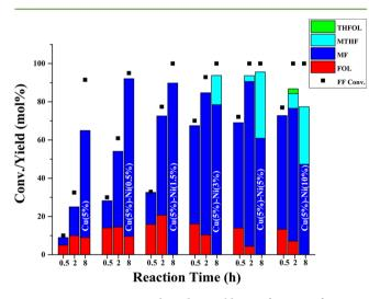
**Figure 4.** FF conversion and product yields as a function of time on  $Cu/TiO_2$  and  $Cu-Ni/TiO_2$  catalysts. The catalyst composition is noted in the 8 h reaction time bar. All reactions were conducted at FF loading of 1 g, catalyst loading of 0.3 g, with 25 mL of 1,4-dioxane as a solvent, and at a temperature of 200 °C. The reactor was pressurized with 35 bar H<sub>2</sub> gas at 25 °C.
