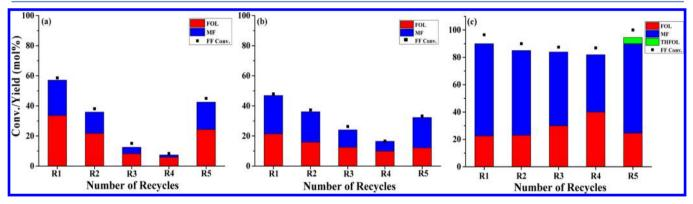
Figure 8. FF conversion and product yields as a function of number of catalyst recycles, R, for (a) Cu/Al<sub>2</sub>O<sub>3</sub>, (b) Cu/TiO<sub>2</sub>, and (c) Cu-Ni/TiO<sub>2</sub> catalysts. After R4, catalysts were calcined at 450 °C for 5 h and reduced at 450 °C for 3 h prior to R5. Reaction conditions were a FF loading of 1 g, catalyst loading of 0.3 g, 25 mL of 1,4-dioxane as a solvent, a temperature of 200 °C, H<sub>2</sub> pressure of 25 bar, and 2 h run time.
