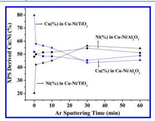
**Figure 3.** Relative Cu/Ni surface concentration (%) for prereduced  $\text{Cu-Ni/TiO}_2$  and  $\text{Cu-Ni/Al}_2\text{O}_3$  catalysts measured by XPS during depth profiling experiments as a function or Ar sputtering time.
