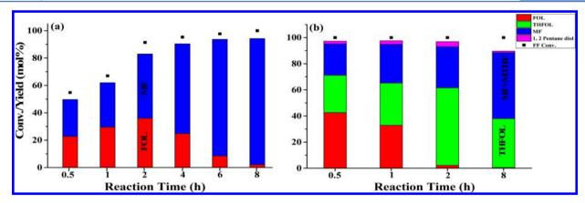
Figure 7. FF conversion and product yields as a function of reaction time over (a) Cu-Ni/TiO<sub>2</sub> and (b) Cu-Ni/Al<sub>2</sub>O<sub>3</sub> catalysts. All reactions were run at a FF loading of 1 g, a catalyst loading of 0.3 g, and 25 mL of 1,4-dioxane as a solvent at a temperature of 200 °C and H<sub>2</sub> pressure of 25 bar.
