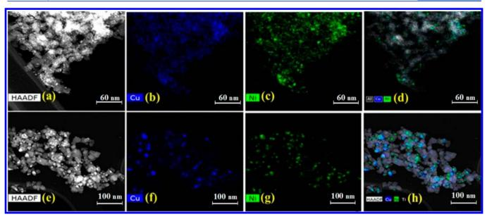
Figure 1. (a) Representative STEM image of the Cu–Ni/Al<sub>2</sub>O<sub>3</sub> catalyst and associated (b) Cu, (c) Ni, and (d) overlaid Cu/Ni/Al elemental mapping. (e) Representative STEM image of the Cu–Ni/TiO<sub>2</sub> catalyst and associated (f) Cu, (g) Ni, and (h) overlaid Cu/Ni/Ti elemental mapping.
