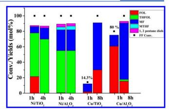
**Figure 6.** FF conversion and product yields over monometallic Ni and Cu supported on  $Al_2O_3$  and  $TiO_2$  catalysts at different reaction times. All reactions were run with an FF loading of 1 g, a catalyst loading of 0.3 g, 25 mL of 1,4-dioxane as a solvent, a temperature of 200 °C, and an  $H_2$  pressure of 25 bar.
