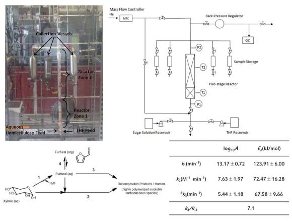
Fig. 4 Reactor schematic, actual reactor and lumped kinetic model for continuous production of furfural in a biphasic reactor. Adapted from ref. 33 and 62.
