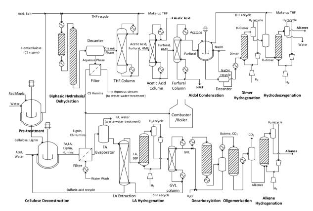
Fig. 13 Simplified process flow diagram for a biorefinery processing red maple as a feedstock for the production of linear hydrocarbons using a hydrolytic fractionation approach
