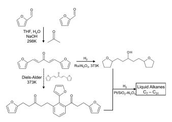
Fig. 5 Overview of chemistry involved in the production of linear and branched alkanes from furfural and acetone.
