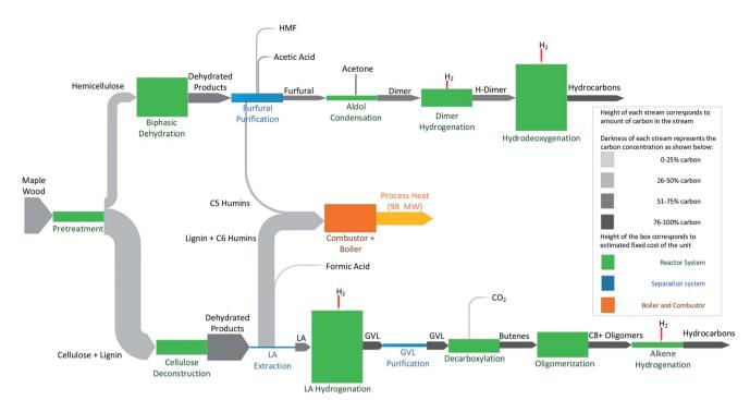
Sankey diagram based on carbon balance of the lignocellulosic biorefinery representing flows of carbon in major streams of the process.
