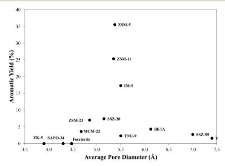
Fig. 10 Aromatic yields as a function of average pore diameter for different zeolites during catalytic fast pyrolysis of glucose in a pyroprobe reactor. Reaction conditions: catalyst-to-feed weight ratio = 19, nominal heating rate 1273 K s<sup>-1</sup>, reaction time 240 s. This figure has been reprinted from Jae, et al. (ref. 95) with permission from the publisher.
