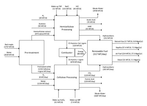
Fig. 14 Overall input-output analysis for different processing units in lignocellulosic biorefinery
