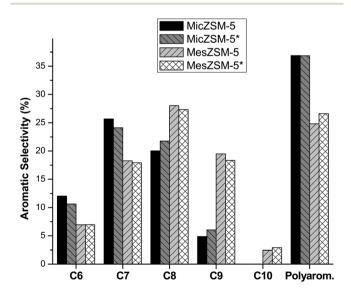
Fig. 11 Distribution of aromatic products from catalytic fast pyrolysis of maple wood over microporous ZSM-5 (MicZSM-5), tartaric acid-treated ZSM-5 (MicZSM-5\*), mesoporous ZSM-5 (MesZSM-5) and mesoporous ZSM-5 treated with tartaric acid (MesZSM-5\*). All studies were carried out using a pyroprobe reactor. Conditions: 873 K, 19 mg catalyst per mg glucose, and 240 s reaction time. Reprinted from Foster, et al. (ref. 94) with permission from the publisher.
