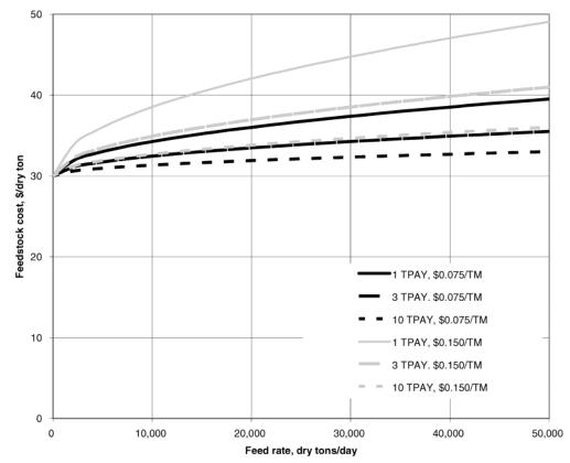
**Figure 1.** Cost of biomass in dollars per dry ton versus amount collected for productivities of 1, 3, and 10 dry tons/acre-year and transportation costs of \$0.075 and \$0.150/wet ton mile with a field cost of \$30/dry ton.
