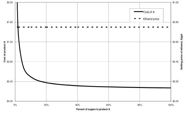
**Figure 6.** Cost of chemical product A in a cellulosic refinery processing 11,025 dry tons/day of cellulosics with a constant ethanol selling price of \$0.75/gal, electricity sold at \$0.05/kwh, and all other parameters as for the base case.
