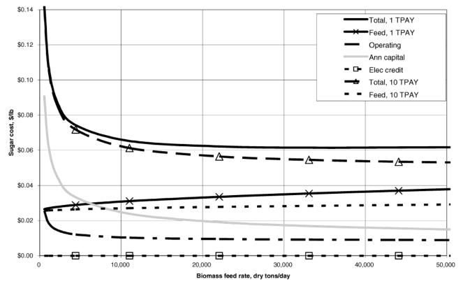
Figure 2. Cellulosic sugar costs for 1 and 10 dry ton/acre-year cellulosic biomass productivities for a field cost of \$30/dry ton, a \$0.125/wet-ton-mile transportation cost, and no electricity sales.
