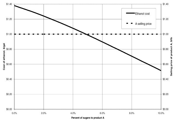
Figure 4. Cost of ethanol for a base case cellulosic refinery with a constant selling price of \$1.00/lb for chemical A and electricity sold at \$0.05/kwh.
