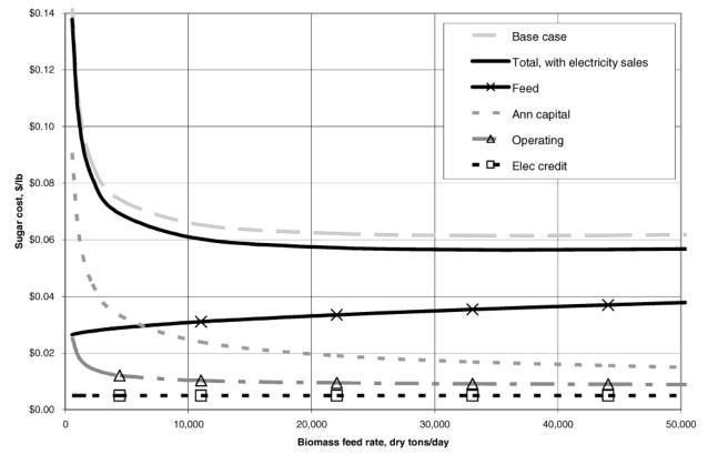
Figure 3. Cellulosic sugar costs for the base case process but with electricity sold at \$0.05/kwh.
