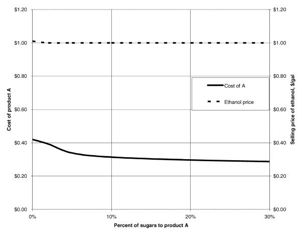
**Figure 5.** Cost of chemical product A in a cellulosic refinery processing 11,025 dry tons/day of cellulosics with a constant ethanol selling price of \$1.00/gal, electricity sold at \$0.05/kwh, and all other parameters as for the base case.
