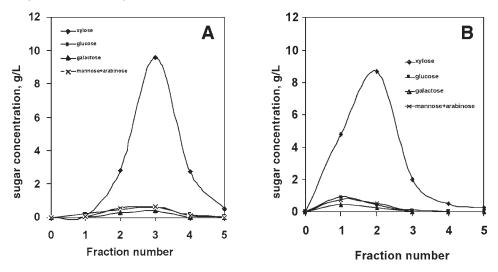
Fig. 4. Sugar concentrations in liquid fractions collected over 4-min intervals for hot water only pretreatment of corn stover at 200°C at velocities of (A) 2.8 cm/min and (B) 10.7 cm/min.
