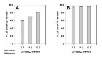
Fig. 6. Monomeric and oligomeric xylose yields for hot water only pretreatment of corn stover at 200°C after (A) 8 min and (B) 16 min.
