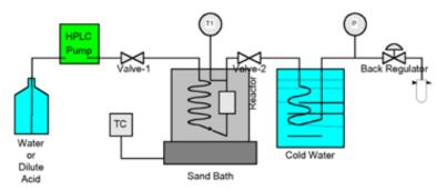
Fig. 1. Schematic diagram of flowthrough system. TC, Thermal controller; T1, thermal couple; P, pressure gauge.
