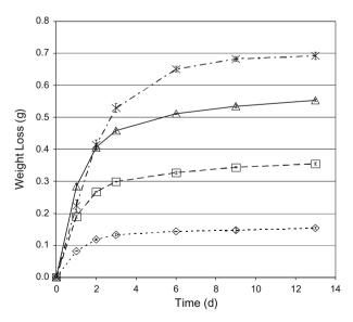
**Fig. 4.** Impact of biomass loading on fermentation results as measured by fermentation bottle weight changes. Soybean hulls SSF with biomass loading of 5%: dots, open diamond; 10%, dashes, open square; 15%, solid line, open triangle, and 20%, dash-dots, X, produced  $8.0 \pm 0.1$ ,  $16.9 \pm 0.1$ ,  $25.2 \pm 0.04$ , and  $32.5 \pm 0.3$  g/L ethanol by day 13, respectively. Spezyme CP®, β-glucosidase dosages were 11 and 13 U/g cellulose, all with SD error bars.
