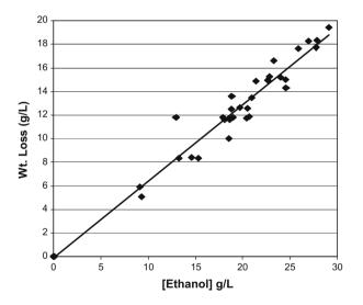
**Fig. 6.** Correlation of weight loss and ethanol concentration for the 30 bottles from Fig. 5, including six zero time samples. Samples are for data from all three ethanologen cultures. Line is a linear calculated fit.
