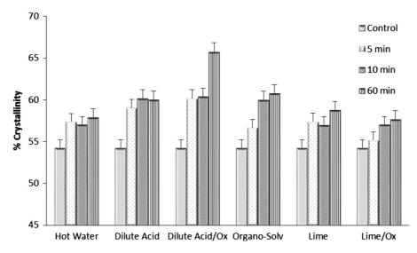
Fig. 4 % Crystallinity of cellulose in the residual pretreated hybrid poplar solids as determined by acid isolated cellulose and <sup>13</sup>C CP/MAS NMR spectra
