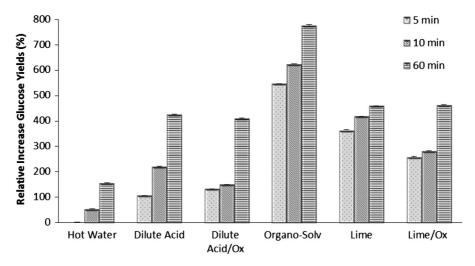
Fig. 5 The relative increase in glucose yields due to enzymatic hydrolysis of pretreated hybrid poplar solids with respect to the sugar release profile of the untreated solids
