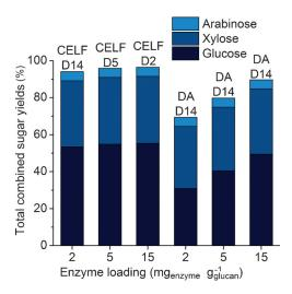
**Figure 4.** Overall Stage 1+Stage 2 yields of glucose, xylose, and arabinose from CELF- and DA-pretreated corn stover solids based on 100 g of total monomeric equivalent of the glucan, xylan, and arabinan content in untreated corn stover. The Stage 2 incubation time in days is shown at the top of each bar, e.g., D14 represents 14 days. 100% corresponds to the maximum amount of sugars that could be realized from the total glucan, xylan, and arabinan in corn stover.
