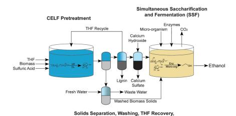
Figure 8. Simplified block flow diagram of a proposed biomass conversion process that integrates CELF pretreatment with SSF to produce ethanol.
