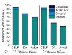
Figure 7. Ethanol yields from SSF of solids from DA and CELF pretreatment of corn stover and Avicel PH-101 cellulose versus culture time at A) 15 mg  $g_{glucan}^{-1}$  and B) 5 mg  $g_{glucan}^{-1}$  loading of Accellerase 1500 enzyme. C) Cumulative yields [%] of SSF metabolites from a seven day culture.
