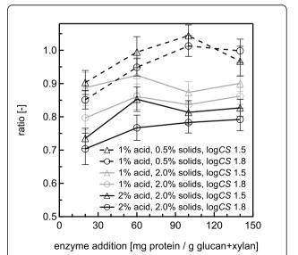
Figure 8 Ratios of sugar yields from co-hydroysis and SPEH for dilute acid pretreatments. Ratios of glucose plus xylose yields from co-hydrolysis to the total yield of these two sugars from SPEH for water-only pretreatment at 140°C of 2% w/w Populus slurries according to the severities and acid concentrations noted for each dataset. The error bars represent the standard errors, based on three replicates.
