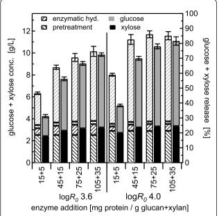
**Figure 4 Hydrothermal pretreatment at 180°C using 2.0% w/w solids concentration**. Glucose and xylose yields from co-hydrolysis compared with those from separate pretreatment and enzymatic hydrolysis (SPEH) for pretreatment of 2% w/w *Populus* slurries in water alone at 180°C followed by enzymatic hydrolysis over a range of enzyme loadings according to the same format as in Figure 2. The error bars represent the standard errors, based on three replicates.
