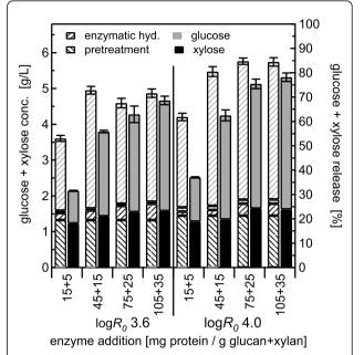
**Figure 3 Hydrothermal pretreatment at 180°C using 1.0% w/w solids concentration**. Glucose and xylose yields from co-hydrolysis compared with those from separate pretreatment and enzymatic hydrolysis (SPEH) for pretreatment of 1% w/w *Populus* slurries in water alone at 180°C followed by enzymatic hydrolysis over a range of enzyme loadings according to the same format as in Figure 2. The error bars represent the standard errors, based on three replicates.
