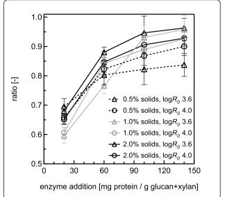
**Figure 5** Ratios of sugar yields from co-hydroysis and SPEH for hydrothermal pretreatments. Ratios of glucose plus xylose yields from co-hydrolysis to the total yield of these two sugars from separate pretreatment and enzymatic hydrolysis (SPEH) for water-only pretreatment at 180°C according to the severities and solids concentrations noted for each dataset. The error bars represent the standard errors, based on three replicates.
