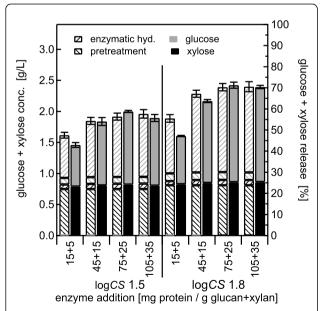
**Figure 9 Dilute acid pretreatment using 1% w/w sulfuric acid** with 0.5% w/w solids concentration. Glucose and xylose sugar yields from co-hydrolysis compared with those from separate pretreatment and enzymatic hydrolysis (SPEH) for pretreatment of 0.5% w/w *Populus* slurries in 1% w/w sulfuric acid at 140°C followed by enzymatic hydrolysis over a range of enzyme loadings according to the same format as in Figure 6. The error bars represent the standard errors, based on three replicates.
