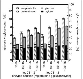
**Figure 7 Dilute acid pretreatment using 2% w/w sulfuric acid** with 2.0% w/w solids concentration. Glucose and xylose yields for co-hydrolysis compared with separate pretreatment and enzymatic hydrolysis (SPEH) for pretreatment of 2% w/w *Populus* slurries in 2% w/w sulfuric acid at 140°C followed by enzymatic hydrolysis over a range of enzyme loadings according to the same format as in Figure 6. The error bars represent the standard errors, based on three replicates.
