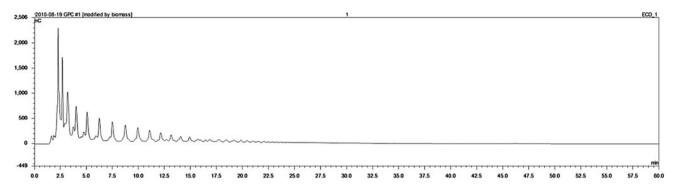
Fig. 2 Example chromatogram from HPAEC-PAD analysis of xylooligosaccharide hydrolyzate produced by hydrothermal pretreatment of birchwood xylan as detected by the Dionex IC system coupled with a CarboPac PA-100 column
