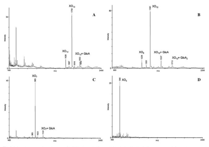
Fig. 5 Selected MALDI-TOF-MS spectra of individual DP xylooligosaccharides isolated by the GPC system: a DP 13, b DP 10, c DP 7, and d DP 4
