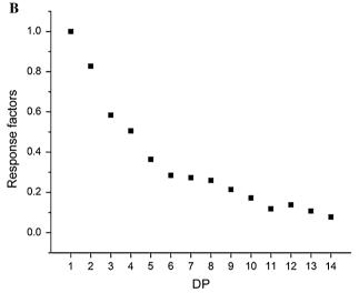
Fig. 7 Response factors based on PAD response peak height (a) and peak area (b) for xylooligosaccharides from DP 2–14, with xylose as the sugar standard
