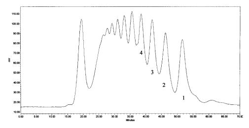
Fig. 3. IMP chromatogram of hydrolysate from uncatalyzed hydrolysis of oat xylan for a 5% solids concentration at 200°C for 10 min. 1, DP1; 2, DP2; 3, DP3; 4, DP4.
