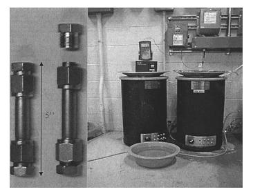
Fig. 1. Tubular reactor system used to hydrolyze xylan.
