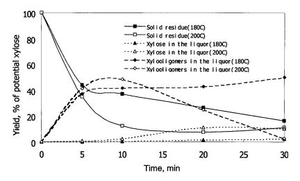
Fig. 2. Sugar recovery for uncatalyzed xylan hydrolysis at 180 and 200°C with 5% solids concentration.
