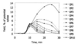
Fig. 5. Oligomer time profiles for uncatalyzed xylan hydrolysis at 200°C with a 5% solids concentration.
