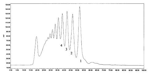
Fig. 4. IMP chromatogram of hydrolysate from uncatalyzed hydrolysis of oat xylan for a 5% solids concentration at 200°C for 20 min. 1, DP1; 2, DP2; 3, DP3; 4, DP4.
