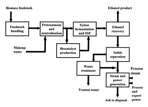
**Figure 1** Block flow diagram for conversion of biomass to ethanol by the NREL process configuration. SSF, Simultaneous saccharification and fermentation.
