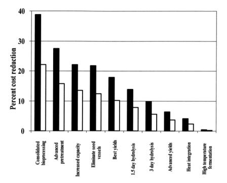
**Figure 4** Impact of advances in key process step configurations and performance parameters on reducing the cost of producing ethanol from biomass based on the advanced-technology scenario. Again, cost reductions compared with the total production cost are shown as *open bars*, whereas the impacts on processing costs alone are presented as *solid bars*.
