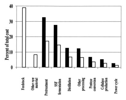
Figure 3 Contribution of major cost elements to overall ethanol production costs for the NREL reference case. Cost reductions based on the total production cost are shown as *open bars*, whereas the impacts on processing costs alone are presented as *solid bars*. SSF, Simultaneous saccharification and fermentation.
