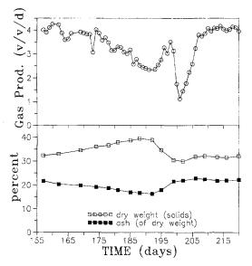
Figure 3. Fermentation performance of one high solids reactor approaching the apparent sludge solids maximum for stable performance of the microbial consortium.
