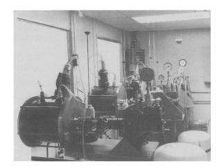
Figure 1. Four bench-scale high solids reactors fed processed MSW. The 20-L cylindrical glass vessels are mixed by agitators driven by individual hydraulic motor assemblies.
