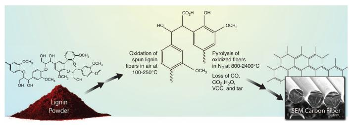
Fig. 4. Highlights of thermal chemistry involved in converting lignin to carbon fiber. See (88, 128) for more information. [Courtesy of Oak Ridge National Laboratory, DOE]
