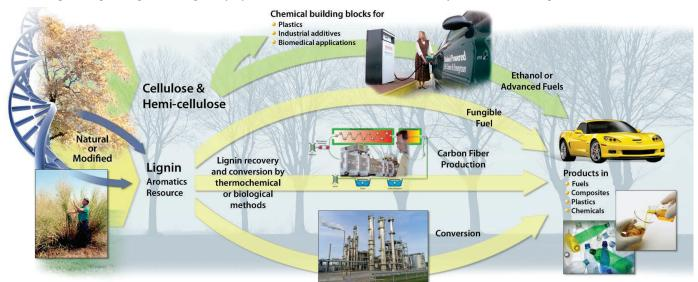
Production of biofuels from cellulosic biomass requires separation of large quantities of the aromatic polymer lignin. In planta genetic engineering, enhanced extraction methods, and a deeper understanding of the structure of lignin are yielding promising opportunities for efficient conversion of this renewable resource to carbon fibers, polymers, commodity chemicals, and fuels. [Credit: Oak Ridge National Laboratory, U.S. Department of Energy]
