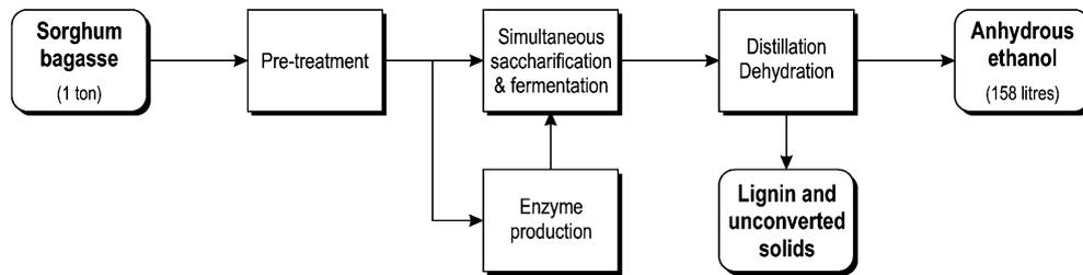
Fig. 7. Block flow diagram for conversion of sorghum bagasse to ethanol.
