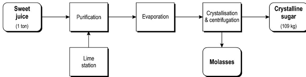
Fig. 5. Block flow diagram for conversion of sweet juice to sugar.
