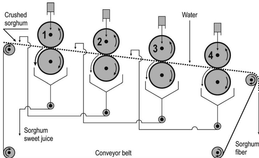
Fig. 3. Schematic diagram of the juice extraction process (adapted from Cundiff et al., 1993).
