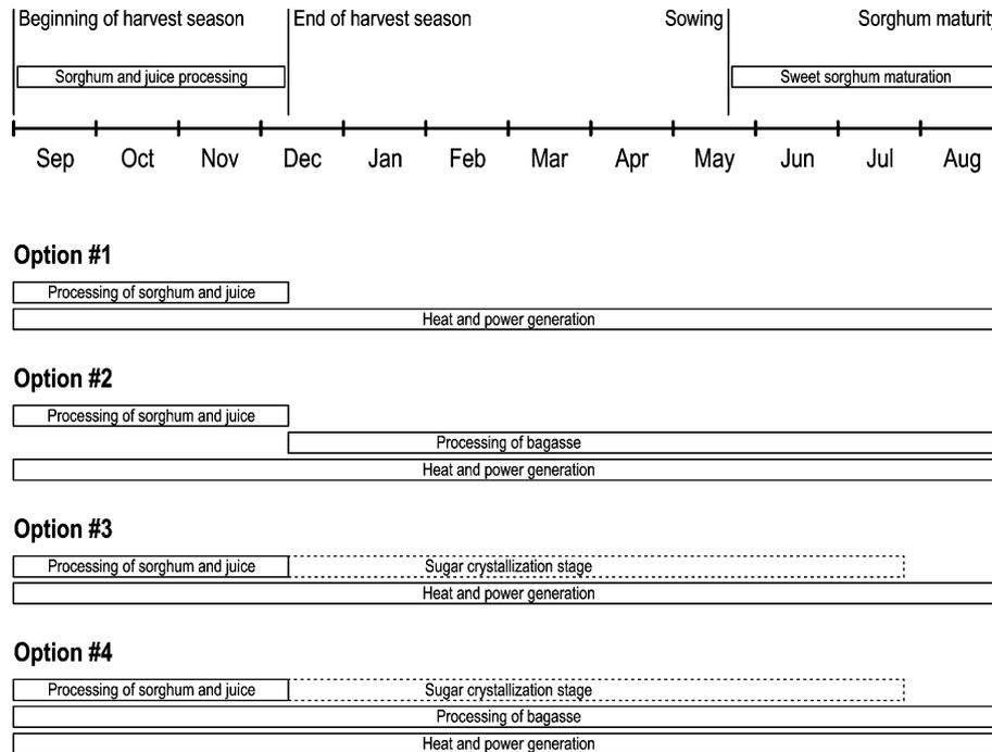
Fig. 2. Time scale and production scheme of the various options.
