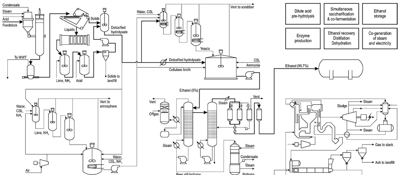
Fig. 8. Schematic representation of the NREL process for ethanol production.
