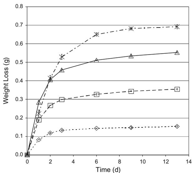
**Fig. 4.** Impact of biomass loading on fermentation results as measured by fermentation bottle weight changes. Soybean hulls SSF with biomass loading of 5%: dots, open diamond; 10%, dashes, open square; 15%, solid line, open triangle, and 20%, dash-dots, X, produced  $8.0 \pm 0.1$ ,  $16.9 \pm 0.1$ ,  $25.2 \pm 0.04$ , and  $32.5 \pm 0.3$  g/L ethanol by day 13, respectively. Spezyme CP<sup>®</sup>,  $\beta$ -glucosidase dosages were 11 and 13 U/g cellulose, all with SD error bars.
