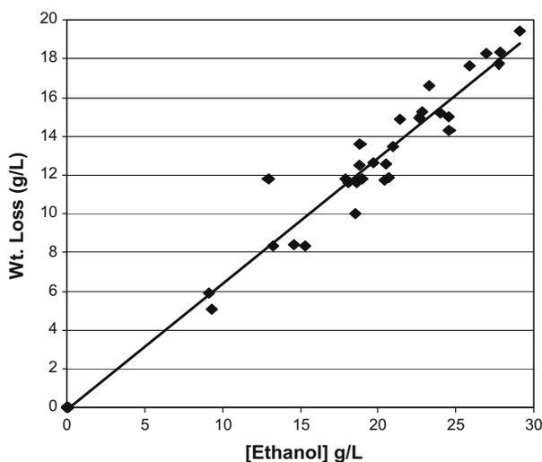
**Fig. 6.** Correlation of weight loss and ethanol concentration for the 30 bottles from Fig. 5, including six zero time samples. Samples are for data from all three ethanologens cultures. Line is a linear calculated fit.
