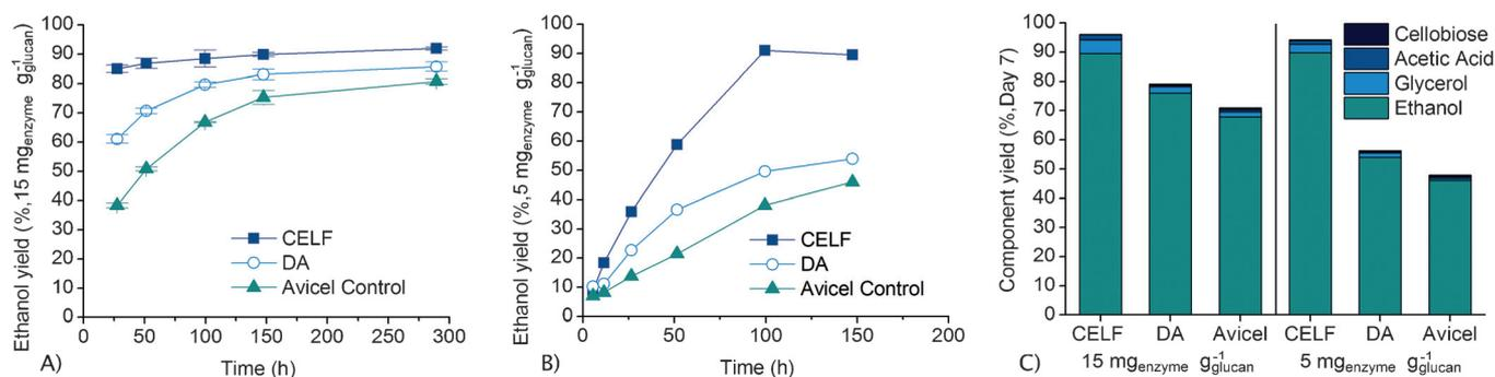
**Figure 7.** Ethanol yields from SSF of solids from DA and CELF pretreatment of corn stover and Avicel PH-101 cellulose versus culture time at A) 15 mg<sub>enzyme</sub> g<sub>glucan</sub><sup>-1</sup> and B) 5 mg<sub>enzyme</sub> g<sub>glucan</sub><sup>-1</sup> loading of Accellerase 1500 enzyme. C) Cumulative yields [%] of SSF metabolites from a seven day culture.
