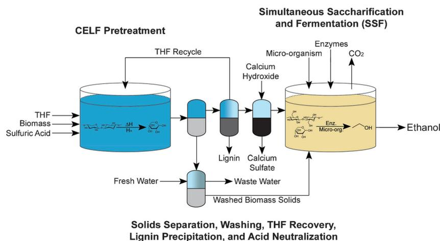
**Figure 8.** Simplified block flow diagram of a proposed biomass conversion process that integrates CELF pretreatment with SSF to produce ethanol.
