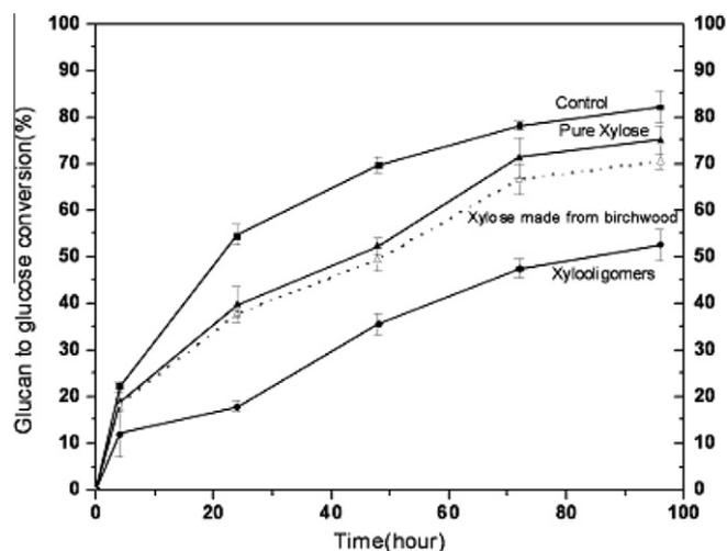
**Fig. 6.** Enzymatic hydrolysis of 2% Avicel with addition of purchased xylose, monomeric xylose made from birchwood, and xylooligomers made by birchwood hydrolysis at an enzyme loading of 5 FPU/g glucan plus 10 CBU/g glucan. All xylose and xylooligomers were added based on equivalent xylose concentration of 5 mg/ml prior to adding enzymes.
