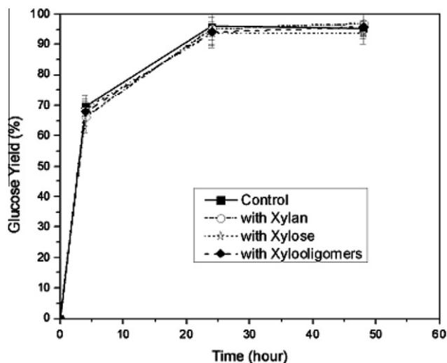
Fig. 3. Enzymatic hydrolysis of 2% cellobiose alone (the control) and with addition of 12.5 mg/ml xylan, mixed xylooligomers, or xylose at a beta-glucosidase loading of 10 CBU/g cellobiose.
