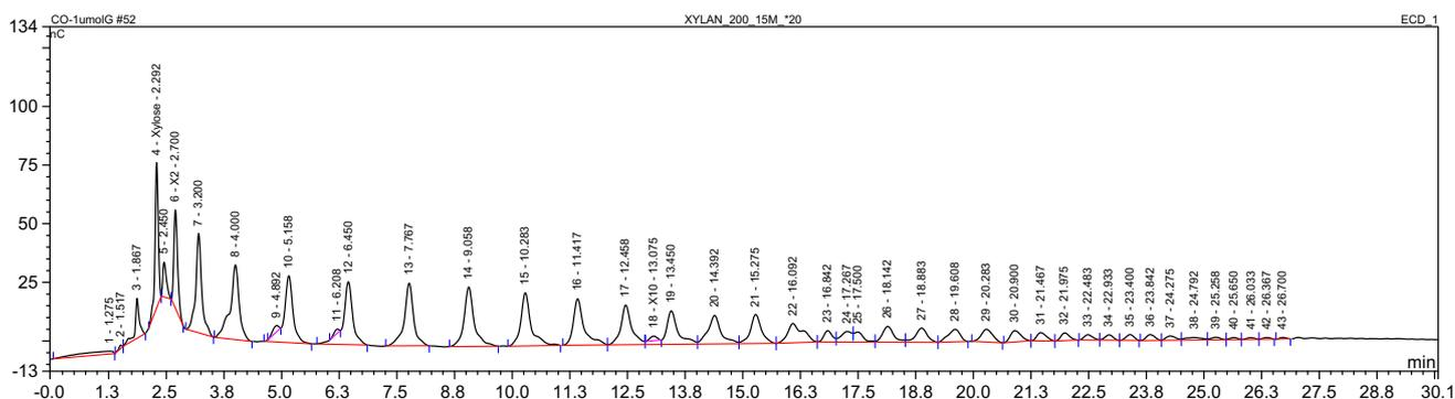
**Fig. 1.** Distribution of the degree of polymerization of soluble xylooligomers produced from xylan as determined by a Dionex IC system equipped with a CarboPac PA100 column.
