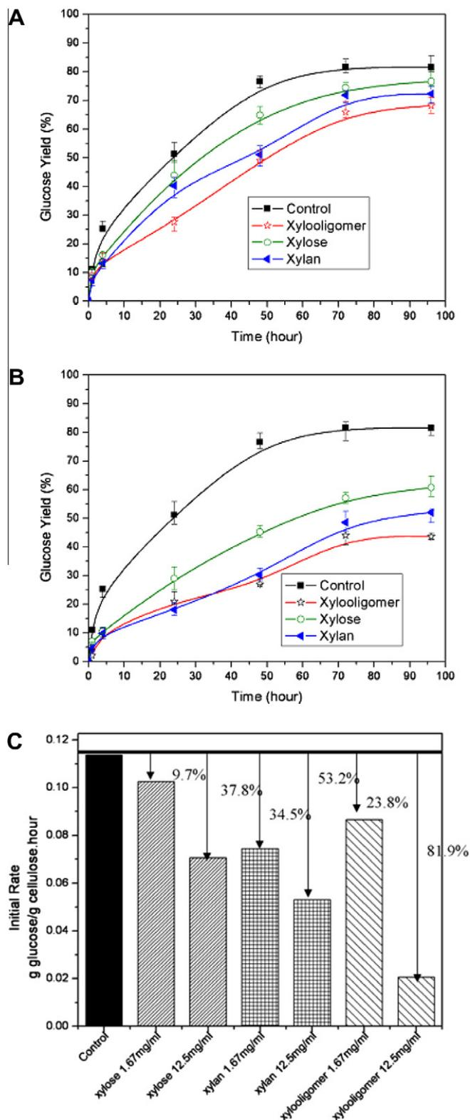
**Fig. 2.** Enzymatic hydrolysis of 2% Avicel alone (the control) and following initial addition of xylose, mixed xylooligomers, or xylan at a mass ratio of 12:1 corresponding to a concentration of 1.67 mg/ml (A) and 12.5 mg/ml (B) of monomeric xylose for an enzyme loading of 5 FPU/g glucan plus 10 CBU/g glucan. Comparison of initial rates of 2% Avicel enzymatic hydrolysis with addition of 1.67 mg/ml and 12.5 mg/ml xylose, mixed xylooligomers, and xylan (C).
