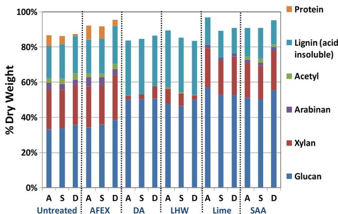
**Fig. 3.** Composition of switchgrass varieties pretreated by leading pretreatment technologies. Untreated switchgrass composition is based on initial dry weight. Pretreated switchgrass composition is based on pretreated solids dry weight. Pretreatment conditions are given in Table 2. Data is average of duplicate analysis. A, Alamo 1; S, Shawnee; D, Dacotah.
