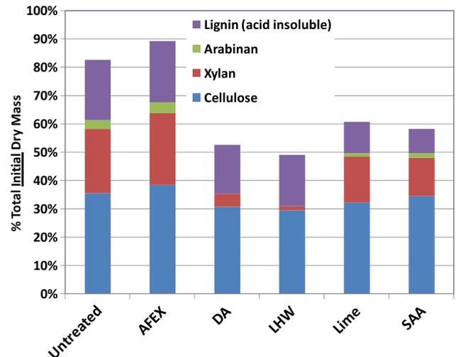
**Fig. 2.** Fate of solids during pretreatment of Dacotah switchgrass. Data is average of duplicate analysis.
