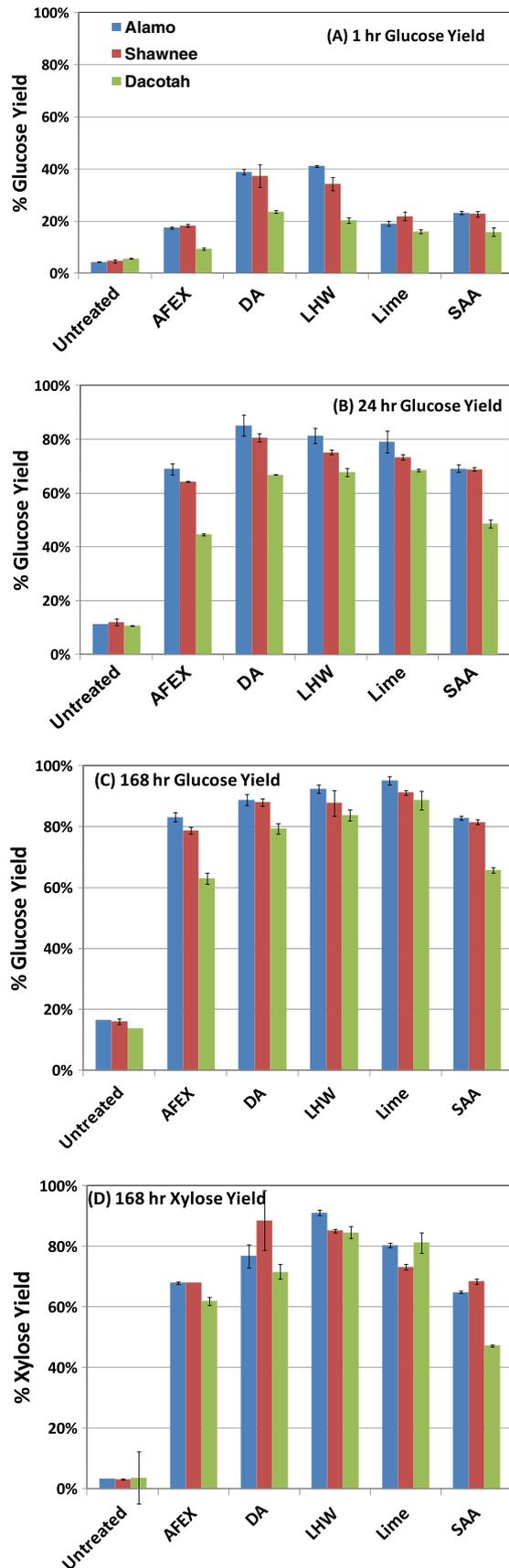
**Fig. 4.** Enzymatic digestibility of switchgrass pretreated by various pretreatment technologies. Pretreatment conditions are given in Table 2. Yields based on glucan or xylan in pretreated/hot washed solids for all pretreatments except for AFEX. Error bars represent 95% CI.
