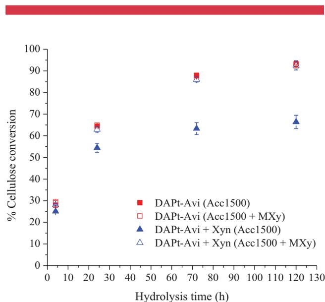
**Figure 3.** Effect of Multifect<sup>®</sup> xylanase (MXy) supplementation (7.5 mg protein/g glucan) of Accellearse<sup>®</sup>1500 (Acc1500) cellulase (15 mg protein/g glucan) on cellulose conversion for washed solids from dilute acid pretreatment (140°C in 1 wt% sulfuric acid for 30 min) of Avicel by itself and mixed with xylan. DAPt- Avi—dilute acid pretreated Avicel cellulose; DAPt- Avi+ Xyn—dilute acid pretreated Avicel mixed with xylan
