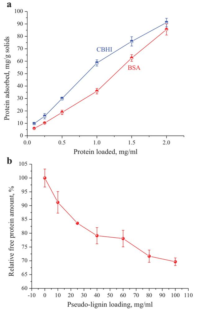
**Figure 8.** a: BSA and purified CBHI protein adsorption on xylose derived-pseudo-lignin (mg/g solids) at a pseudo-lignin solids loading of 10 g/L. b: Effect of pseudo-lignin loading on relative amount of free BSA protein in solution for a BSA loading of 2 mg/mL.
