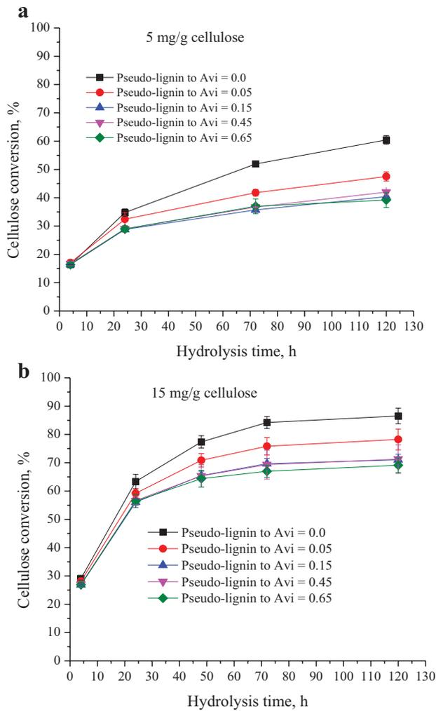
**Figure 7.** Effects of various levels of exogenously added pseudo-lignin on cellulose conversion at cellulase protein loadings of (a) 5 mg/g cellulose and (b) 15 mg/g cellulose.
