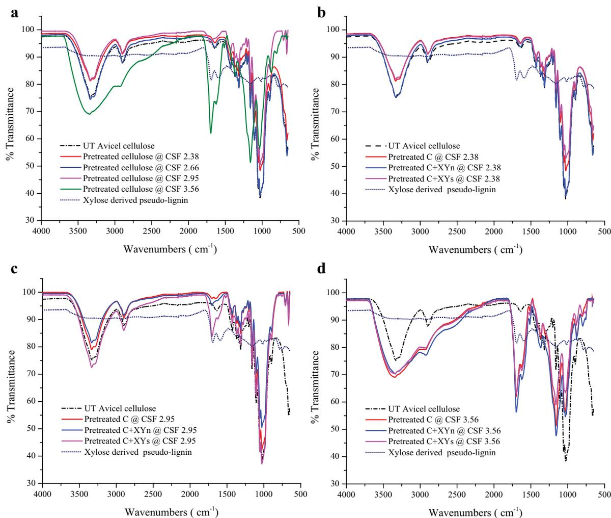
**Figure 5.** FT-IR spectra of untreated and dilute acid pretreated Avicel PH 101 cellulose prepared at various severities, and comparison with spectra for xylose derived-pseudo-lignin and dilute acid pretreated Avicel cellulose alone and when mixed with xylan or xylose: (a) untreated, (b) CSF 2.38, (c) CSF 2.95, and (d) CSF 3.56.
