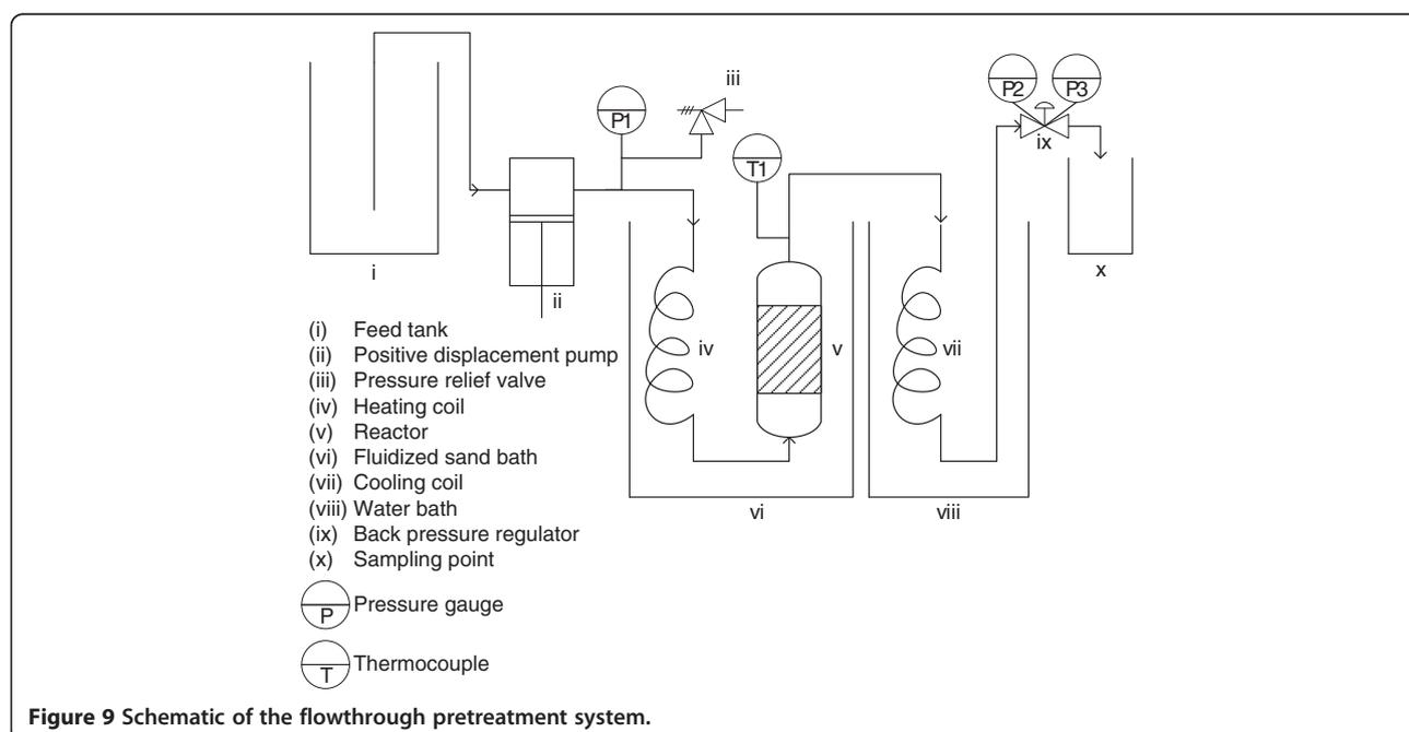
**Figure 9 Schematic of the flowthrough pretreatment system.**
