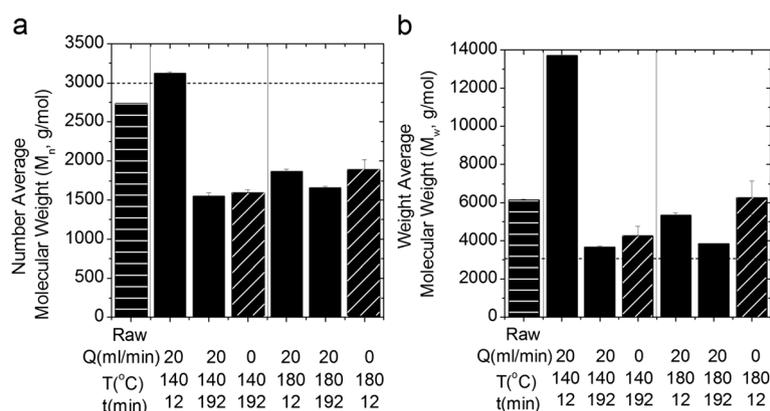
**Figure 3** Molecular weights of cellulolytic enzyme lignin (CEL) as determined by gel permeation chromatography: (a) number average and (b) weight average. Molecular weights of CEL before pretreatment, after flowthrough pretreatment, and after batch pretreatment are shown with horizontal hatching, solid, and diagonal hatching, respectively. The black dashed line represents a molecular weight of 3000 on both panels.
