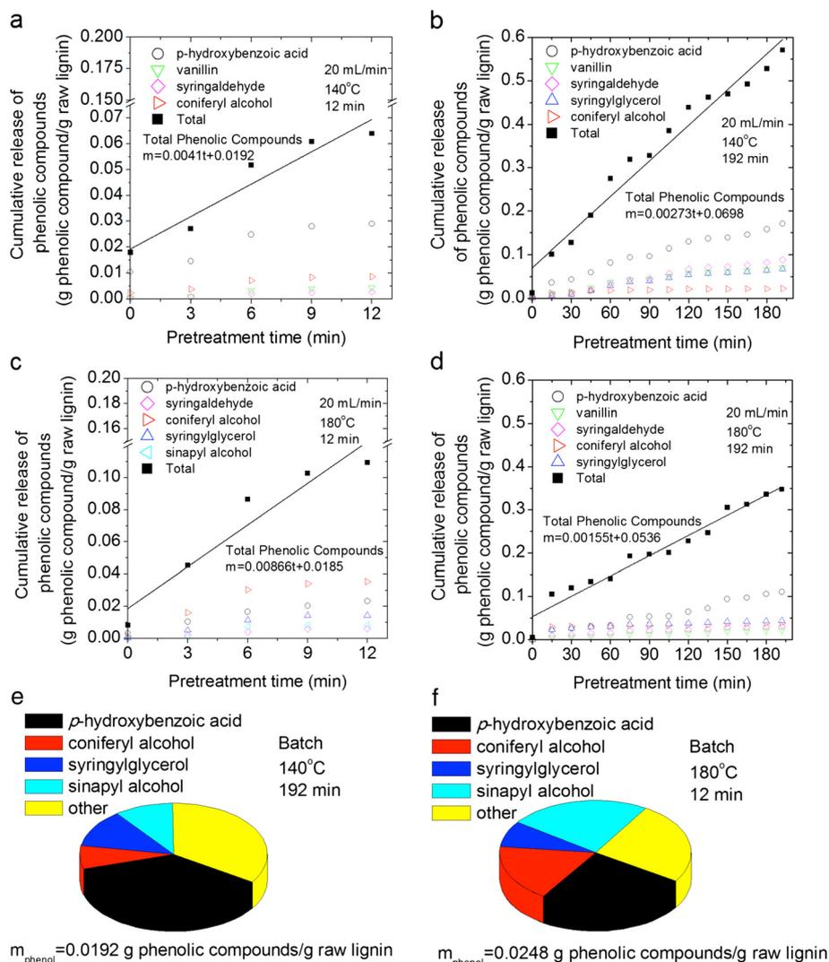
**Figure 8** Phenolic compounds in hydrolysate generated by flowthrough and batch pretreatment of *Populus trichocarpa* x *P. deltoides* wood samples. Cumulative release of phenolic compounds from flowthrough pretreatment (20 mL/min) are plotted as a function of time: (a) 140°C, 12 min; (b) 140°C, 192 min; (c) 180°C, 12 min; (d) 180°C, 192 min. Distribution of primary phenolic compounds after batch pretreatment: (e) at 140°C for 192 min and (f) at 180°C for 12 min.
