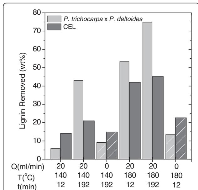
**Figure 6** Percent lignin removal from *Populus trichocarpa*  $\times$  *P. deltoides* wood samples and cellulolytic enzyme lignin (CEL) after batch (0 mL/min, diagonal hatching) and flowthrough (20 mL/min, solid) pretreatments at 140 and 180°C for 12 and 192 minutes. Percent lignin removal was calculated from the Klason lignin and total solids mass balance. See Additional file 1, Additional file 2, Additional file 3, and Additional file 4 for details of the calculations.
