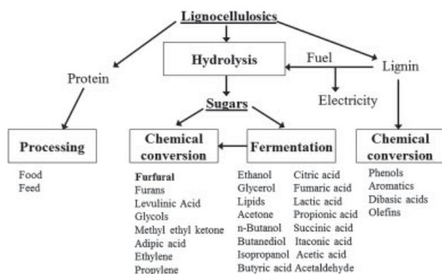
**Figure 2.** Conversion of sugars, lignin, and protein in lignocellulosic biomass for the integrated production of fuels, chemicals, materials, heat, power, food, and feed. (Adapted from Wyman.<sup>36</sup>)
