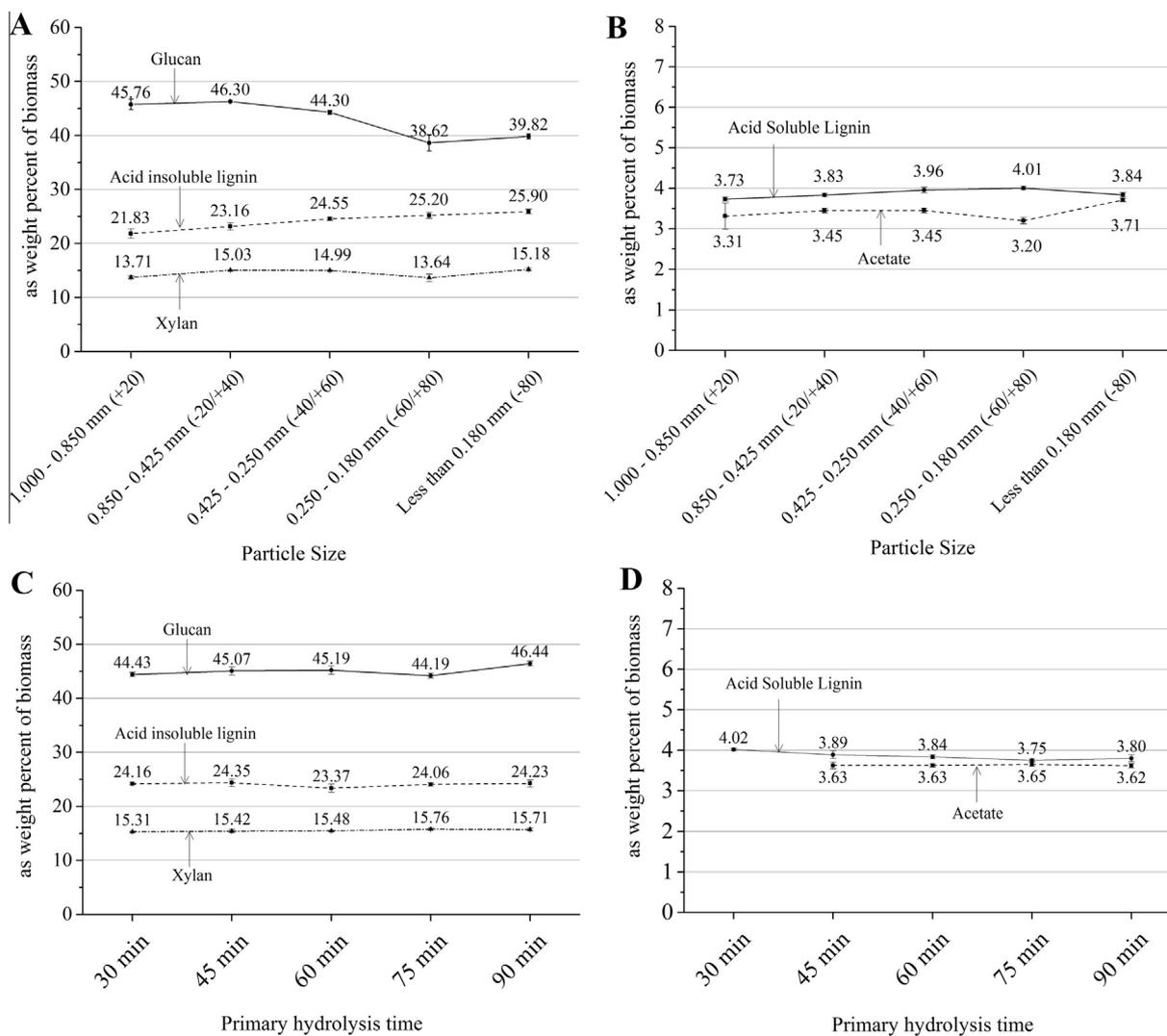
**Fig. 2.** Effect of particle size and primary hydrolysis time on composition. (A) Shows glucan, xylan and AIL contents whereas (B) shows acetate and ASL contents with variation in particle size. (C) Shows glucan, xylan and AIL contents whereas (D) shows acetate and ASL contents with variation in primary hydrolysis time. Error bars represent standard deviation from three replicates.
