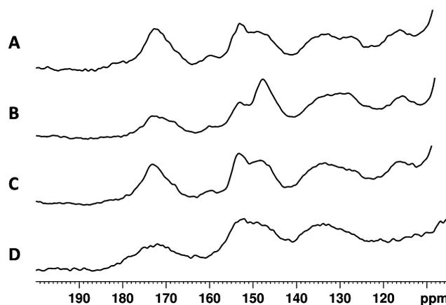
**Fig. 6** Aromatic region of solid-state <sup>13</sup>C cross polarization magic angle spinning (CP/MAS) spectra of switchgrass feedstock before and after conversion. (A) Switchgrass feedstock before conversion. (B) Residue after hydrothermal pretreatment. (C) Residue remaining after *C. thermocellum* fermentation. (D) Residue remaining after *C. thermocellum* cotreatment following removal of metal particles by sonication after suspension in an EDTA solution.
