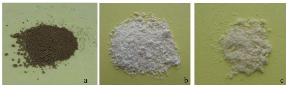
**Fig. 1** Representative images of isolated lignin, cellulose and hemicellulose from diluted acid pretreated poplar (pretreatment at 26.8 min). a: lignin; b: cellulose; c: hemicellulose.
