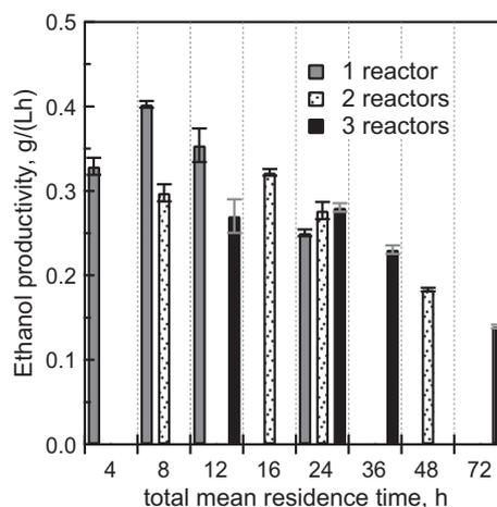
**Fig. 6.** Average ethanol productivities from continuous simultaneous saccharification and fermentation (cSSF) of dilute acid pretreated corn stover solids for each stage in the 3-stage train. Samples were taken from each fermentor for separate runs at each residence time of 4, 8, 12 and 24 h per reactor, resulting in the displayed set of 12 steady state concentrations.
