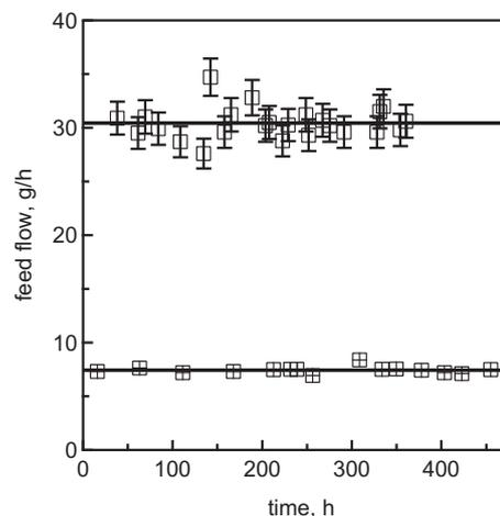
Fig. 2. Targeted and measured feed flow rates. The lower data are for feeding Avicel at a residence time of 96 h, and the upper data are for feeding corn stover for a residence time of 24 h. The solid lines represent the target flow rates. The error bars for corn stover correspond to  $\pm 5\%$  of the measured feed rate. No error bars are shown for the Avicel feed.
