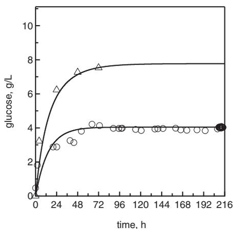
**Fig. 3.** Glucose concentrations measured for batch ( $\Delta$ ) and 24 h residence time continuous ( $\circ$ ) enzymatic hydrolysis of Avicel cellulose at 50 °C with a 1% w/w cellulose loading as well as the corresponding modeling predictions (solid lines) for an enzyme loading of 10 FPU ( $\text{g}_{\text{glucan}}^{-1}$ ).
