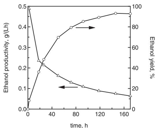
**Fig. 4.** Ethanol yield and productivity for batch SSF of dilute acid pretreated corn stover at a cellulose loading of 2% (w/w) and a temperature of 38 °C with an enzyme loading of 5 FPU  $\text{g}_{\text{glucan}}^{-1}$ .
