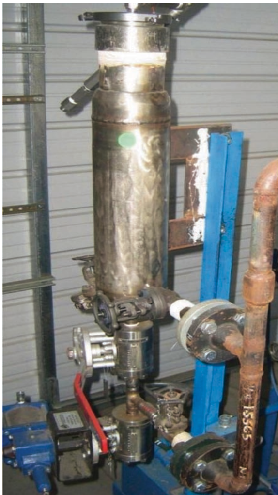
Fig. 4. Steam gun pretreatment reactor system.
