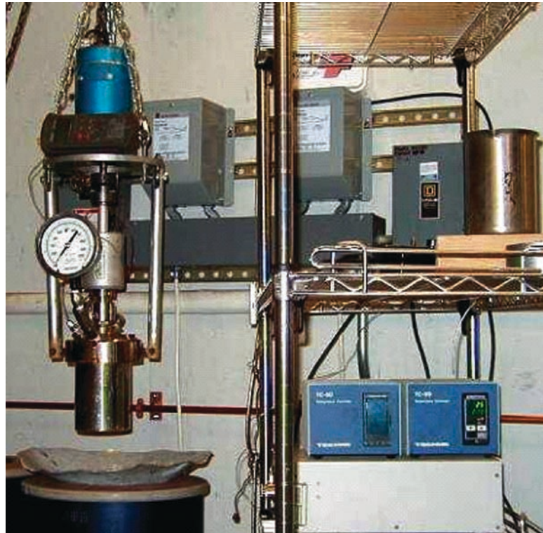
Fig. 2. Mixed Parr reactor pretreatment and fluidized sand bath system.
