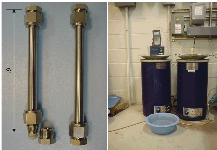
Fig. 1. Batch tube reactors and fluidized sand bath system.
