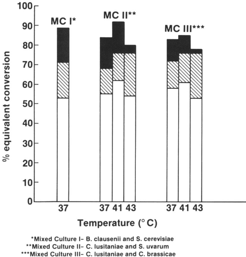
Fig. 7. Comparison of the percent equivalent cellulose conversions for mixed cultures at selected temperatures with Genencor 150 L cellulase enzyme at a loading of 13 IU/g of 10% Sigmacell 50 substrate after 2 d (□), 4 d (▨), and final day (■).
