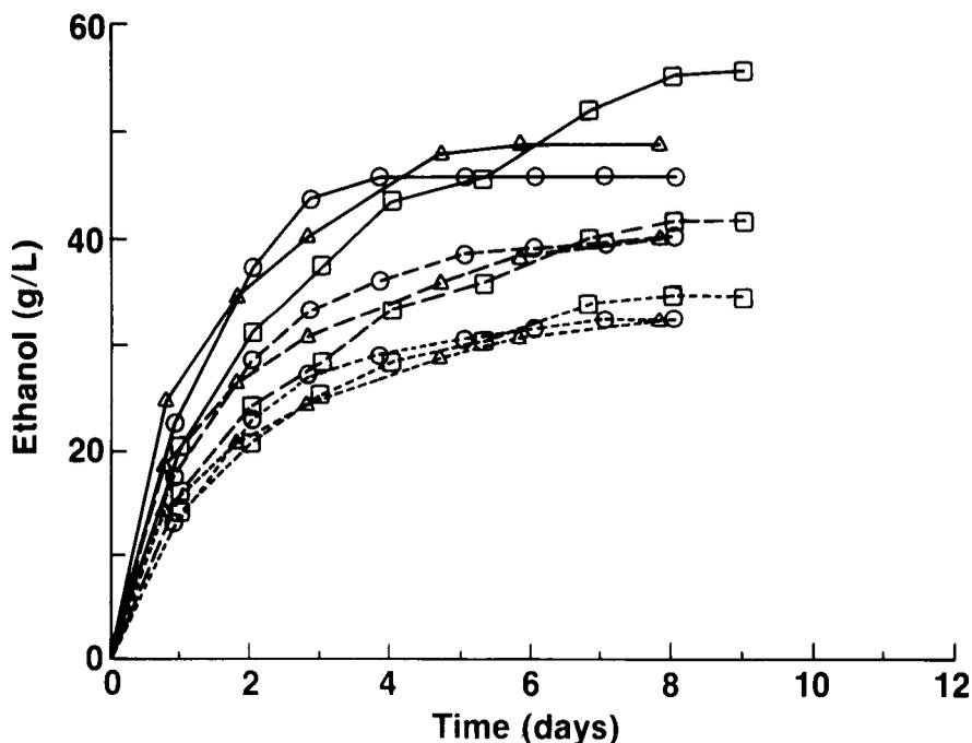
Fig. 3. Ethanol production in small scale SSF experiments for *S. uvarum* with Genecor 150 L cellulase enzyme at 37 (□), 41 (△), and 43°C (○). Enzyme loadings are 13 IU/g Sigmacell 50 cellulose substrate at 7.5 (---), 10 (-.-), and 15% (-) w/v.
