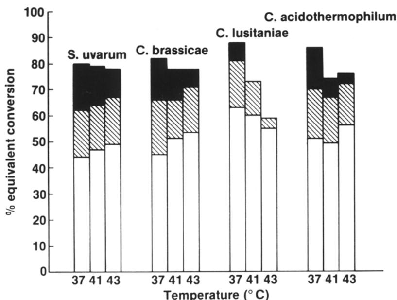
Fig. 6. Comparison of the percent equivalent cellulose conversions for four thermotolerant yeasts at selected temperatures with Genencor 150 L cellulase enzyme at a loading of 13 IU/g of 10% Sigmacell 50 cellulose substrate after 2 d (□), 4 d (▨), and final (■).
