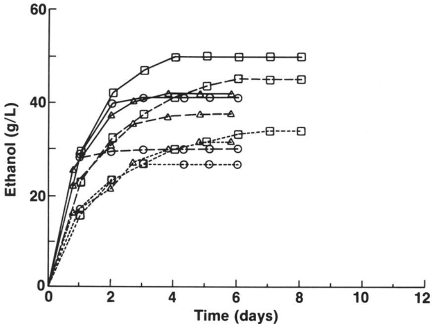
Fig. 4. Ethanol production in small scale SSF experiments for *C. lusitaniae* with Genecor 150 L cellulase enzyme at 37 (□), 41 (△), and 43°C (○). Enzyme loadings are 13 IU/g Sigmacell 50 cellulose substrate at 7.5 (---), 10 (—), and 15% (· ·) w/v.
