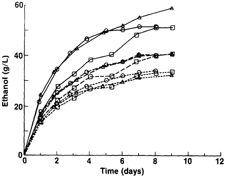
Fig. 1. Comparison of Genecor 150 L saccharification at 30 ( $\diamond$ ), 37 ( $\square$ ), 45 ( $\circ$ ), and 50°C ( $\triangle$ ) at cellulase loading of 26 IU/g with Sigmacell 50 cellulose at 10 (closed) and 15% (open) w/v.
