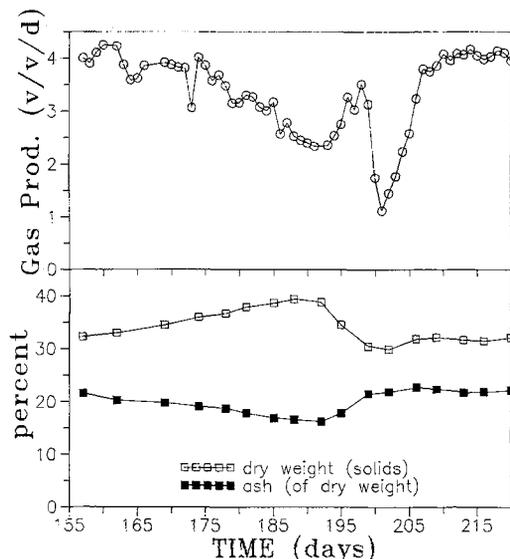
Figure 3. Fermentation performance of one high solids reactor approaching the apparent sludge solids maximum for stable performance of the microbial consortium.
