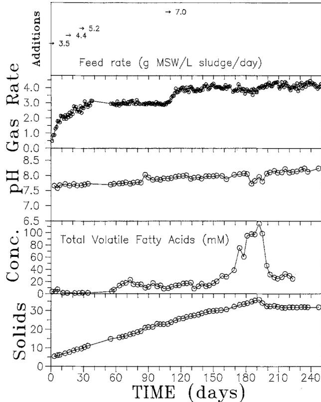
Figure 2. Fermentation performance for high solids anaerobic digestion of MSW through gradual solids buildup. Data represents the average of four high solids reactors operated in parallel. Gas production shown is in volumes of biogas per volume of sludge per day. Volatile fatty acid pools reflect the total for C2-C5 iso- and normal acids. Sludge solids concentration were determined on a dry weight basis (wt/wt).
