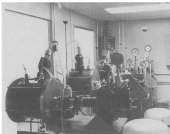
Figure 1. Four bench-scale high solids reactors fed processed MSW. The 20-L cylindrical glass vessels are mixed by agitators driven by individual hydraulic motor assemblies.
