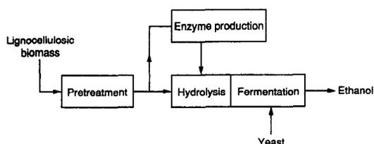
Fig. 1. The simultaneous saccharification and fermentation (SSF) process combines cellulose hydrolysis to glucose and fermentation of glucose to ethanol in one vessel.
