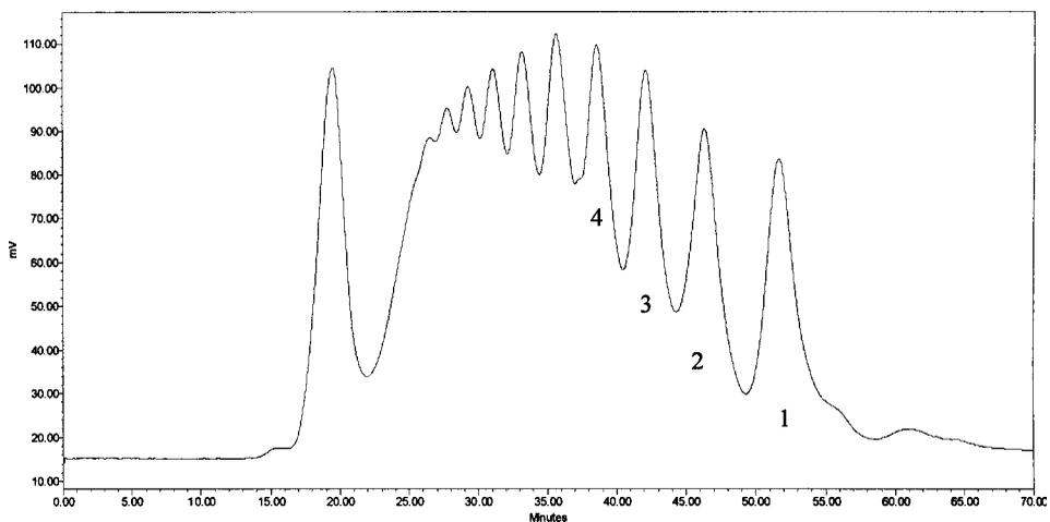
Fig. 3. IMP chromatogram of hydrolysate from uncatalyzed hydrolysis of oat xylan for a 5% solids concentration at 200°C for 10 min. 1, DP1; 2, DP2; 3, DP3; 4, DP4.
