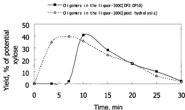
Fig. 6. Total oligomer yields determined by IMP and posthydrolysis.
