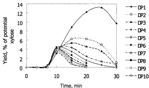
Fig. 5. Oligomer time profiles for uncatalyzed xylan hydrolysis at 200°C with a 5% solids concentration.
