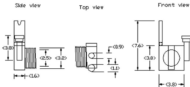
**Figure 2.** Schematic representation of the small in situ device including a side view, top view, and front view. All the units are in centimeters.
