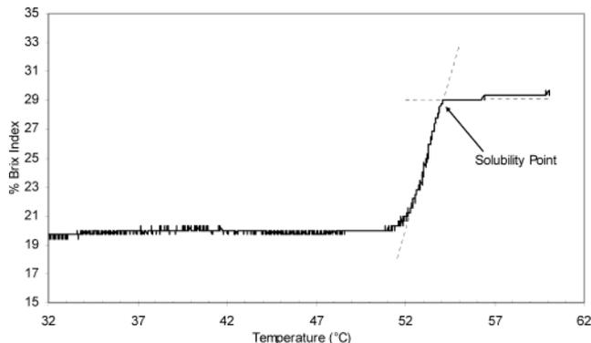
**Figure 4.** Change in refractive index with temperature for the larger in situ device with an initial solids loading of 0.067 27 g of sugar/g of total mass. The solubility point is the point at which the line changes from a sharp climb to being almost horizontal, indicating the dissolution of all solids.
