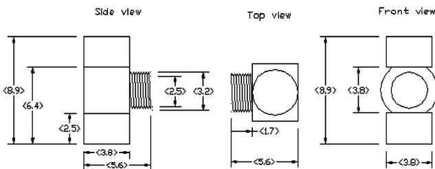
**Figure 1.** Schematic representation of the large in situ device including a side view, top view, and front view. All the units are in centimeters.
