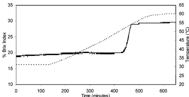
**Figure 3.** Continuous recording of the sample refractive index (solid line) and temperature (dotted line) versus time for the larger in situ device. The initial solids loading was 0.067 27 g of sugar/g of total mass.
